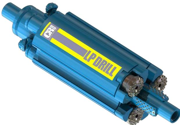
The Mining LP is really today's version of the LP used for the Chilean Mine Rescue. These tools are specially designed for angled holes, utilizing a stinger with a pilot hole to guide the Mining LP. Special features have been designed into the unit to ensure applicability to the harsh, underground mining environment. Mining LP's are used to create burn holes, utility holes, ventilation, dewatering, and rescue shafts from 20" (508mm) to 120" (3048mm).
