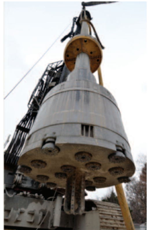
Anatomy of a reverse circulation LP Canister Drill. The 12-inch, carbide button stinger of this 72-inch LP Canister Drill isn't meant to drill but to follow the initial pilot hole. Its interchangeable hammers will be removed for use in the 108- and 132-inch hole openers that follow. The weighted centralizer on the drill string contributes to the stability of the rotating drill.
