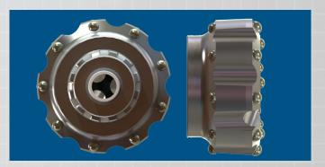
**Back Reamer**, designed for use in unstable rock drilling conditions where operator has to back ream to remove tools from hole. The back reaming inserts protect the bit body from wear and damage when grinding out of hole.
