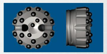
**Concave/Convex (X)**, the best of both worlds with double gauge row and concave center for medium to hard and abrasive formations, straight holes, excellent flushing and excellent penetration rates.
