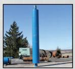
Center Rock's can rods and hammer shrouds are used to fill the annular space between the hole being drilled and the drill tools to increase up-hole velocity for hole cleaning instead of adding additional air compressors.
